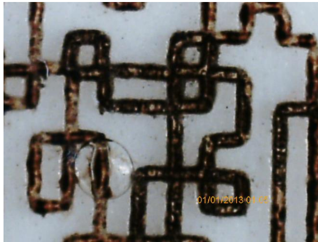
Figure 11: Sheet of 3% w/w Glycerol and 3% w/w alginate after it was engraved by the Epilog laser
