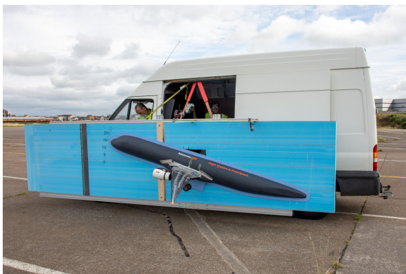
(a) Van-Test used as makeshift wind tunnel [16].
