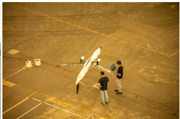
(b) Tether-Test for handling characteristics [16].
