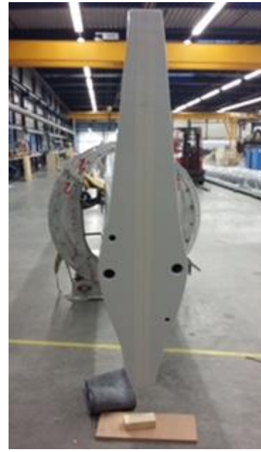
Assembled Mast Top Plate
