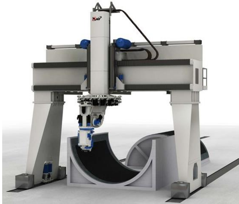
Figure 22: ATL Process Set-up on a Gantry Crane
