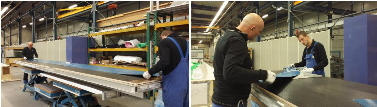
Figure 17: Laminating Process of a Flat Plate
