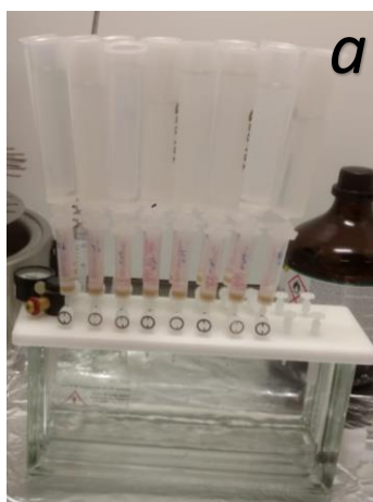
Figure 6: a: filling the reservoirs with the sample, b: removing the analytes from the cartridges, c: nitrogen evaporator.
