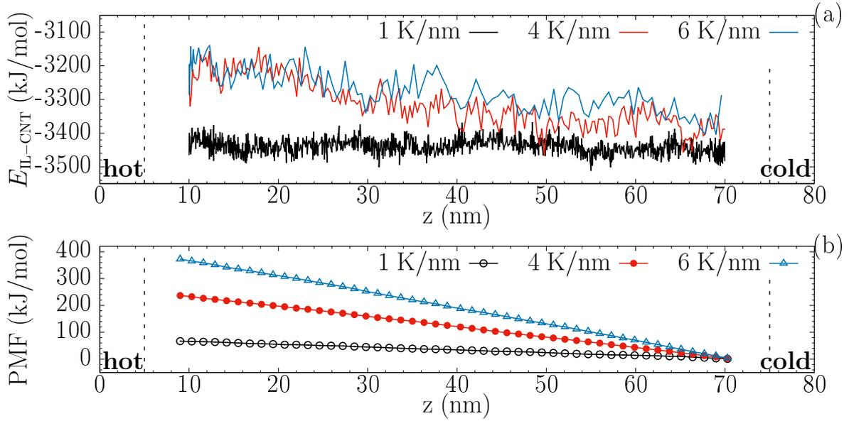
**Figure 3.** (a) Interaction potential energy of between the droplet and CNT as the droplet move from hotter to colder region along the nanotube axis. (b) Potential of mean force of the droplet against its centre-of-mass position.
