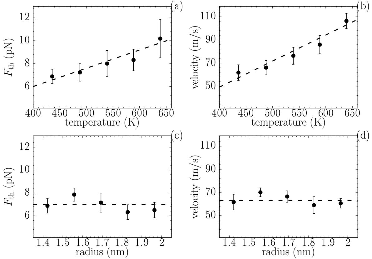
**Figure 8.** Variation of the thermophoretic force and the terminal velocity as a function of the average system temperature ((a) and (b)) and the radius ((c) and (d)) of the CNT, respectively at a constant thermal gradient of 4 K/nm. The dashed lines indicate a linear fit of the data.
