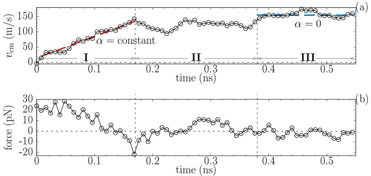
**Figure 4.** Change in (a) the velocity of centre of mass of droplet and (b) force acting on IL droplet over time. Region I, II and III (in (a)) show the acceleration phase with a constant slope ( $\alpha$ ), transient phase and steady phase with a constant speed, respectively.
