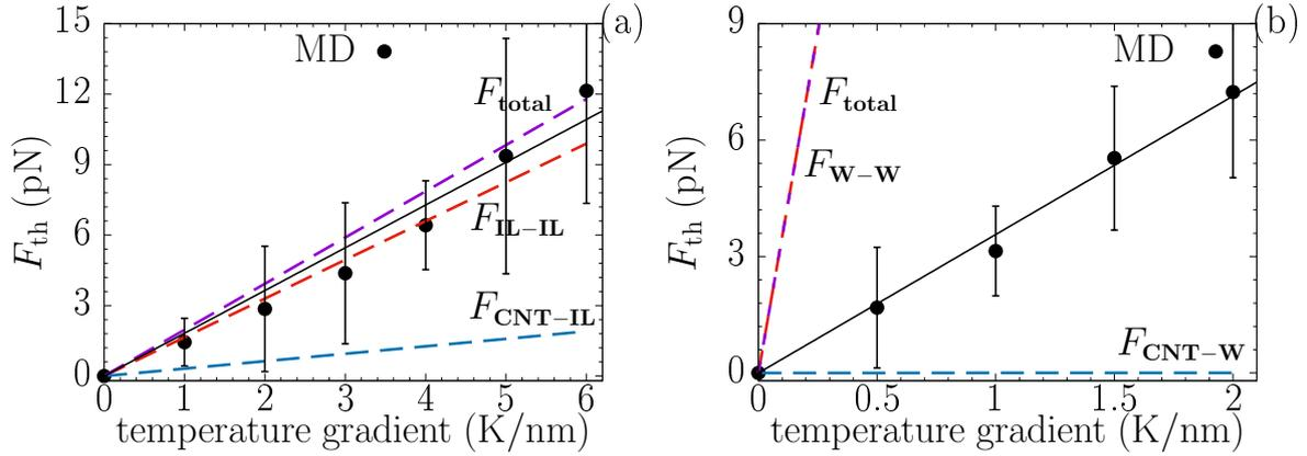
**Figure 6.** Thermophoretic forces with the temperature gradient for (a) the IL and (b) the water droplets. Filled circles denote results calculated from the acceleration phase in the nonequilibrium simulations. Dashed lines denote the forces calculated from the theoretical approach (Eq. 4), based on the variation in potential energy with temperature in Fig. 5.
