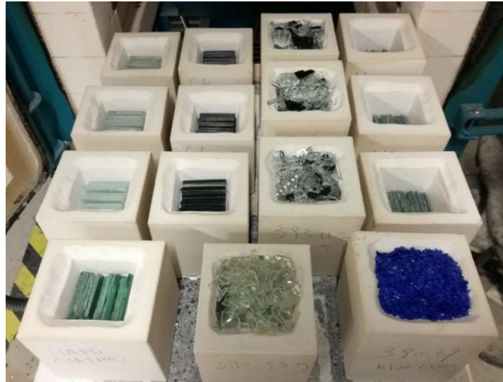
Fig. 1: Arrangement of glass cullet in disposable silica plaster moulds
