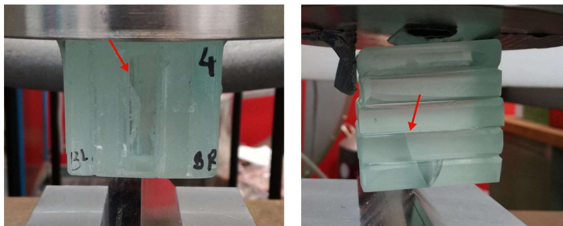
Fig. 22: Float specimens glued with DELO and tested in parallel (left) or perpendicular (right) orientation. In the left case, the crack will propagate throughout the specimen and move along the adhesive layer once it reaches it, while in the right case, the propagation will be completely arrested by the adhesive interface
