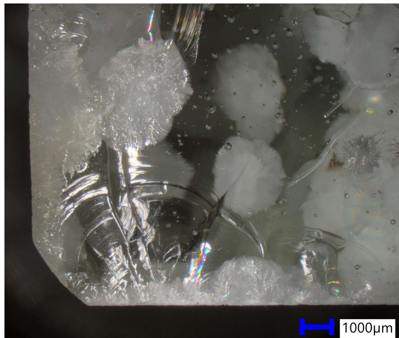
Fig. 24: Fracture origin of a heat-treated “Clear bottle cullet” specimen, showing the interchange between glassy and crystalline material at the process zone of the crack
