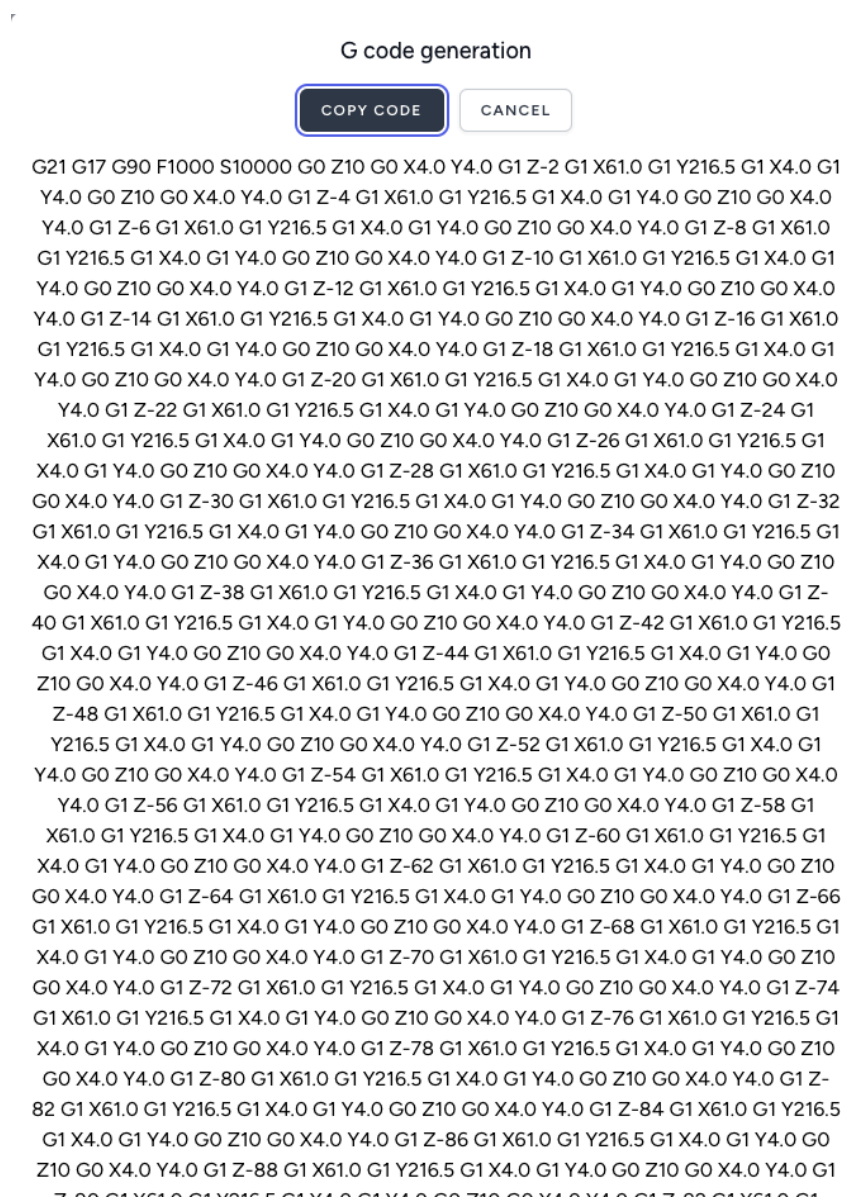
Figure 4.17: G-code generated and sent to CNC-provider order box
