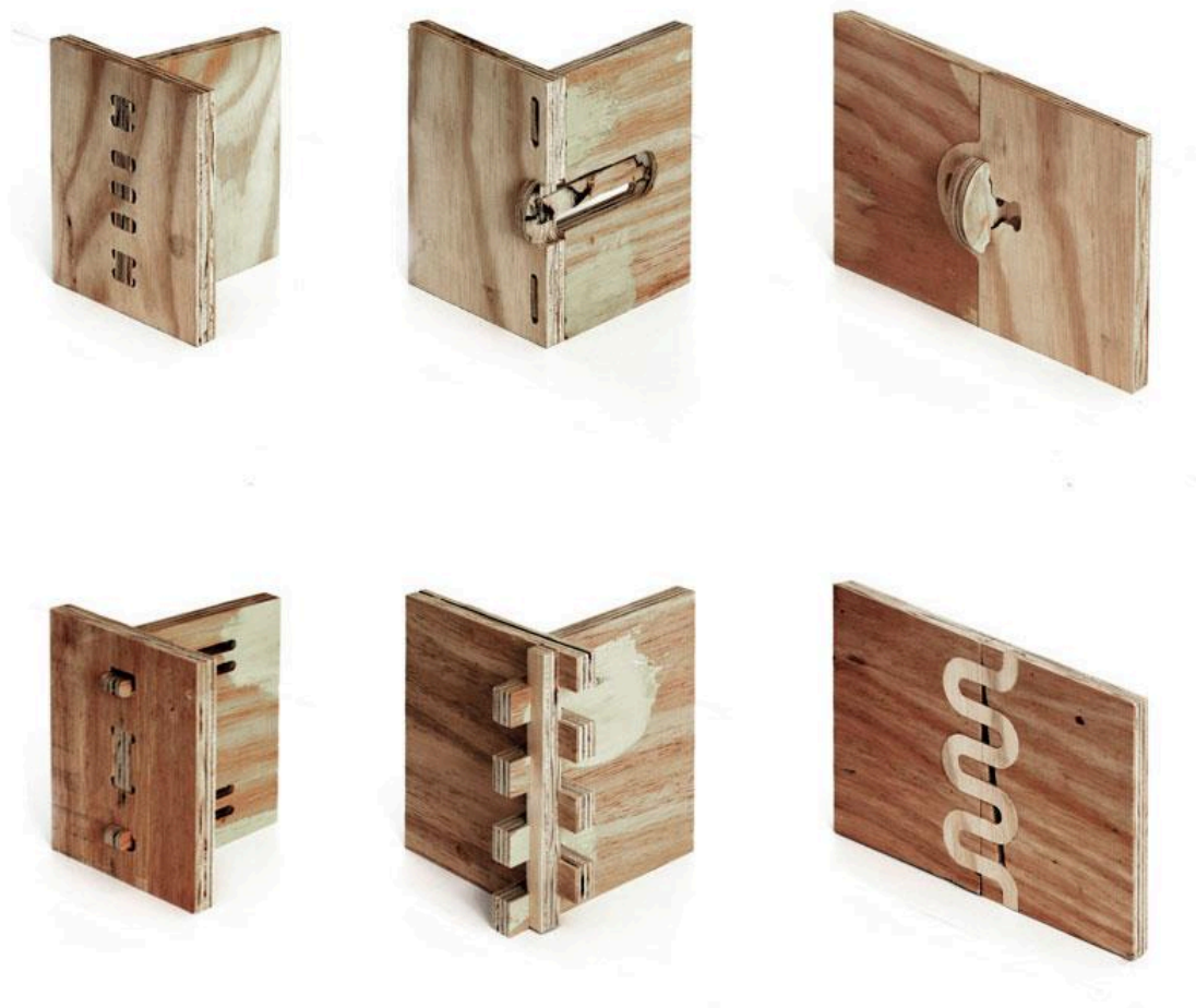
Figure 2.5: Haiti's 5-Hour Emergency Shelter, each section has a different kind of interlocking part
