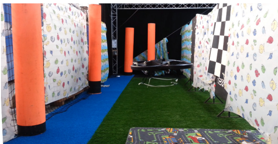
Fig. 14. 'Corridor' environment inside the Cyberzoo. The corridor is a rectangular area of approximately 10 \times 3 m. Shower curtains have been placed along the sides of the corridor to provide sufficient texture for navigation.
