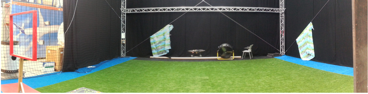
Fig. 11. TU Delft's Cyberzoo , a 10 \times 10 \times 7 m testing area for UAVs. To provide additional texture for visual homing, the left curtain is partially opened and shower curtains are hung on the back- and right walls.
