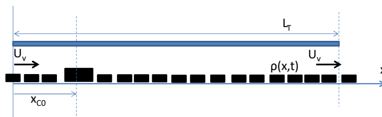
Figure 3.1 Schematic of the considered scenario where an accident is caused by a truck at position x_{c0} in a traffic jam.
