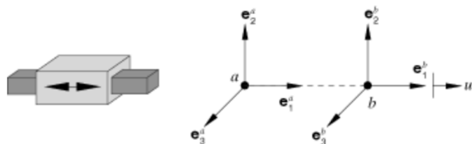
Figure 4.9: Connection type TRANSLATOR imposes kinematic constraints and uses local orientation definitions equivalent to combining connection types SLOT and ALIGN [11]
