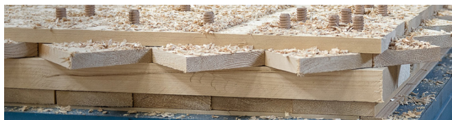
The production process of dowel laminated timber (StructureCraft, 2019)
