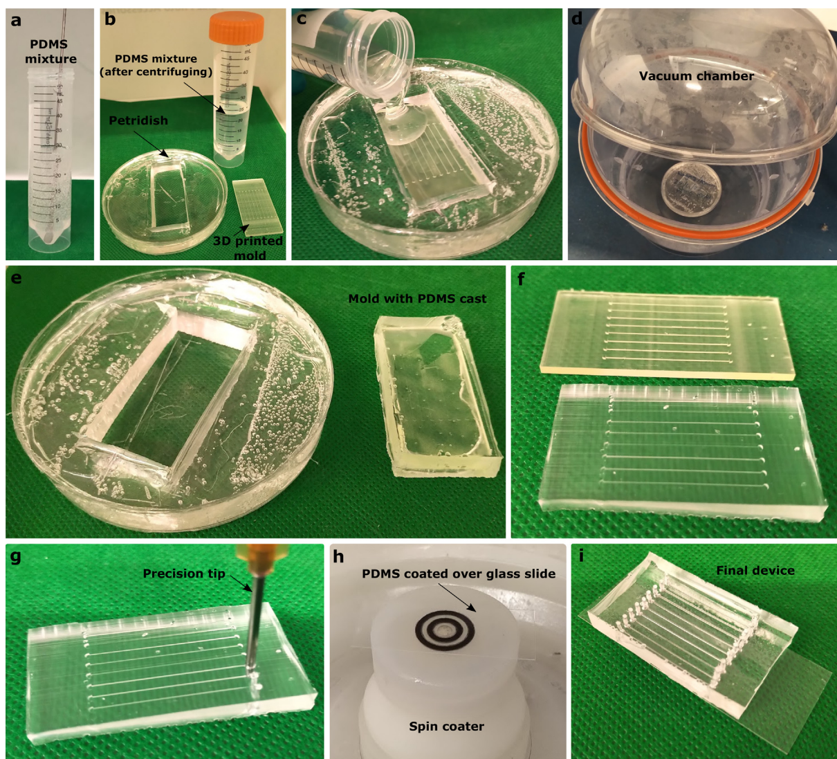
Fig. 5. Visual demonstration of the fabrication procedure of microchannels. a) PDMS mixture is prepared. b) 3D printed mold is placed inside the petridish. c) The centrifuged PDMS mixture is poured into the petridish containing the mold. d) Vacuum is applied to remove the air bubbles present. e) PDMS is cured together with the mold and the required portion of PDMS along with the mold is cut carefully after curing. f) PDMS cast is separated from the mold. g) Inlet and outlet ports are created using the precision tip. h) A layer of PDMS is spin-coated over the cover glass. i) Coated cover glass is bonded with the PDMS cast to obtain the final device.
