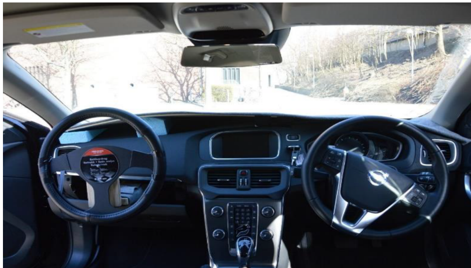
Figure 6.1: Inside of Wizard-of-Oz vehicle [33]
