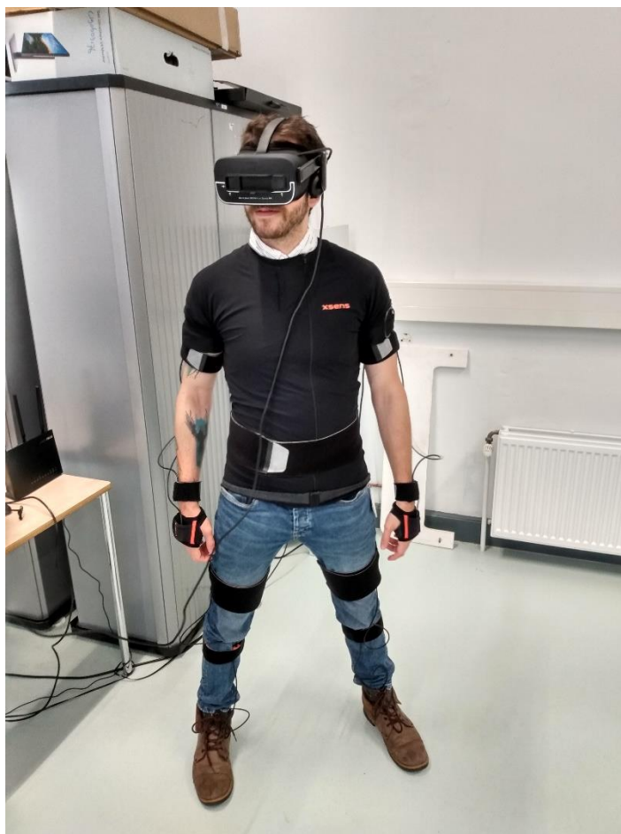
Figure 1: Participant wearing Xsens Link and Oculus Rift
