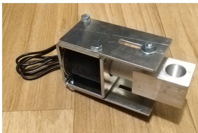
Figure 4.13: View of the droplet catcher
