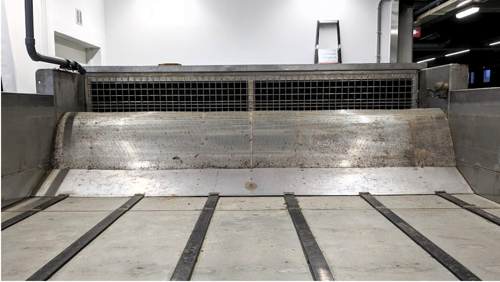
Figure 2.6: Beach that was designed to dissipate waves at the end of the test section
