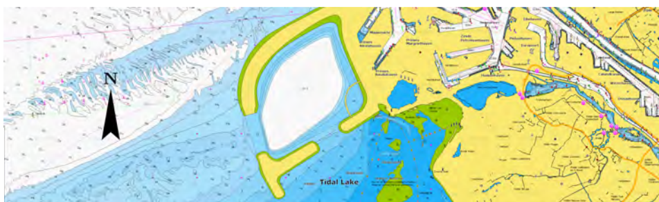
Figure 7.6: Step 3: Construction of the Southern Dunes Connecting the Spillway, Barrier and Pumping Station
