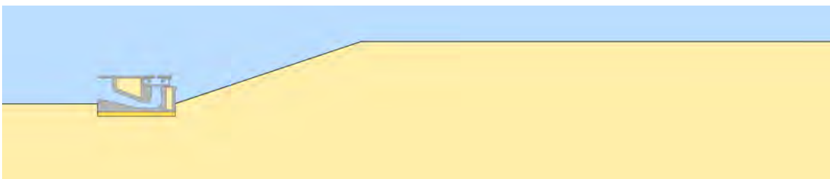
Figure U.7: Backfilling around pumphouse
