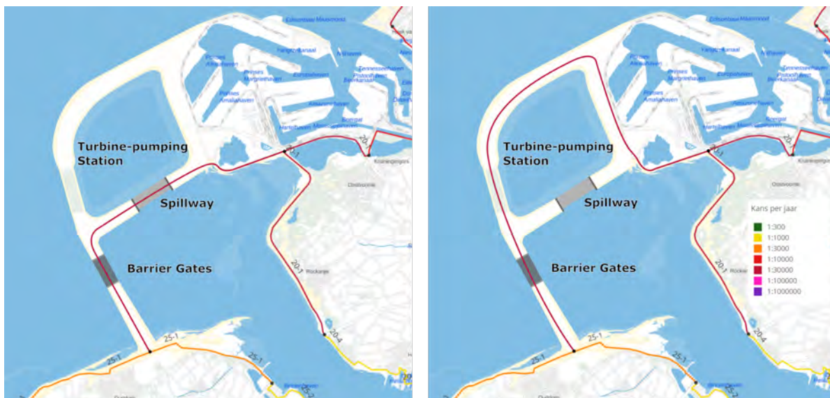
Figure 4.1: Connection of the Delta21 Elements to the Current Primary Flood Defense System (Red Line)
