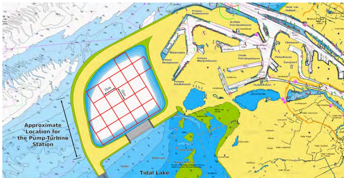
Figure 3.1: Spatial Design of the Energy Storage Lake and Approximate Location of the Pump-turbine Station
