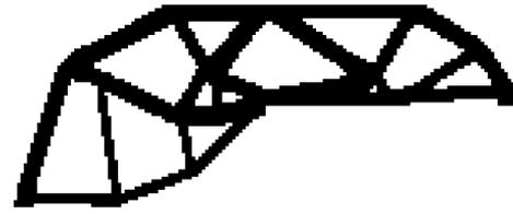
Fig. 4. The binary image based on the TO result.
