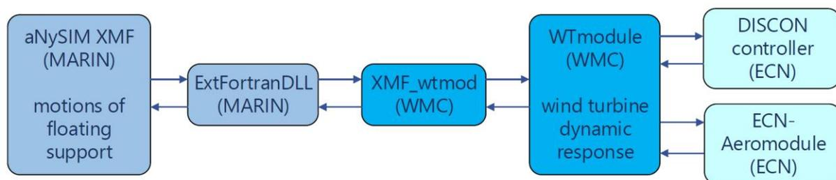
**Figure 6.** Coupled software for floating VAWT analysis
