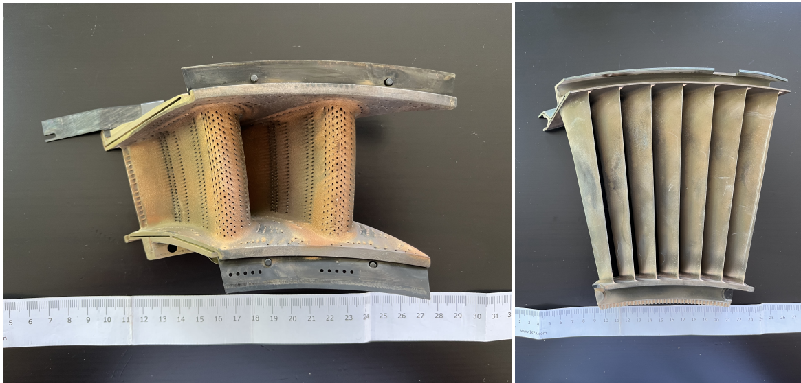
Figure 4.11: CFM56-5C nozzle guide vanes (left) and stage 4 LPT stator vanes (right).
