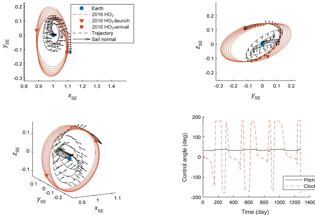
**Fig. 9** Solar-sail case—optimized trajectory and controls for ideal sail model and  $\beta = 0.025$ .
