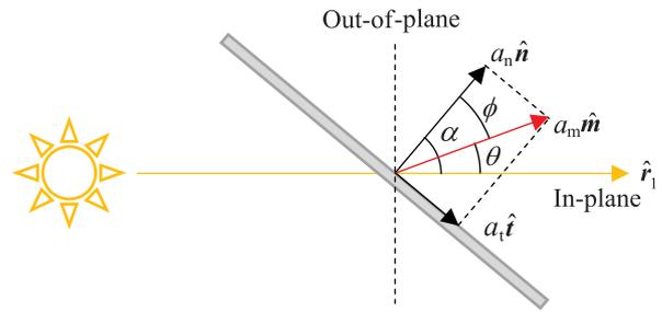
Fig. 3 Side-view schematic of non-ideal solar-sail acceleration components.
