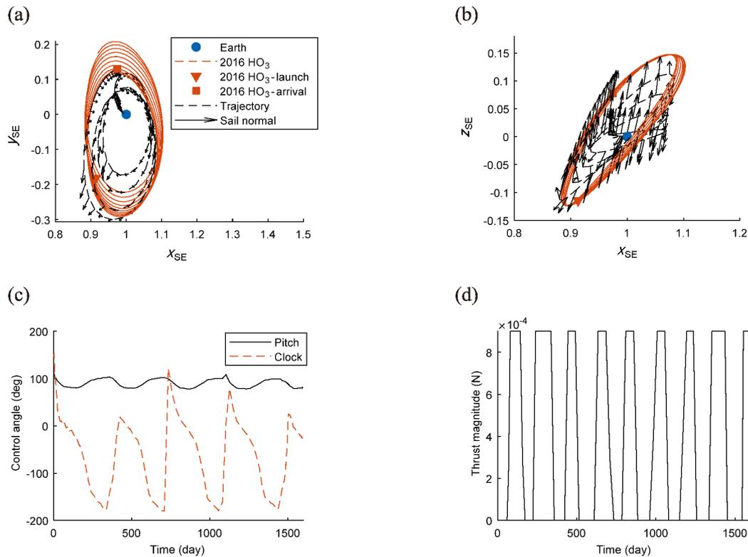
**Fig. 11** SEP case—minimum-propellant results for case 1:  $m_0 = 14$  kg,  $I_{sp} = 1600$  s, and  $T_{max} = 0.9$  mN. (a) Trajectory projected onto the ecliptic plane. (b) Trajectory in the out-of-plane direction. (c) Thrust angles. (d) Thrust magnitude.
