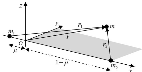
Fig. 2 Schematic of circular restricted three-body problem.
