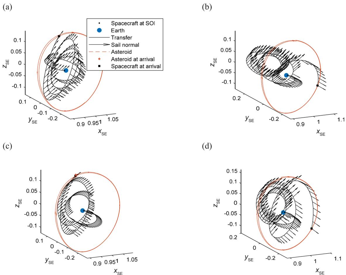
**Fig. 7** Solar-sail case—best initial guess trajectories in the synodic Sun–Earth frame  $B_{SE}(x_{SE}, y_{SE}, z_{SE})$  for an ideal solar-sail model and for (a)  $\beta = 0.025$ , (b)  $\beta = 0.03$ , (c)  $\beta = 0.035$ , and (d)  $\beta = 0.04$ .
