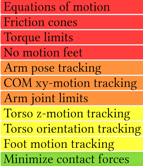
Figure 4.2: Task hierarchy including arm joint limits. Tasks are grouped and ordered from high (red) to low (green) priority. The extra priority level (orange) will result in torso motion to accommodate the end-effector motion tracking task when one of the arm joint limits is activated.
