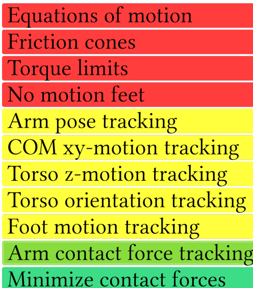
Figure 6.1: Task hierarchy including end-effector contact force control task. The additional priority level at which this task is placed guarantees that when this task will only be executed as well as is possible without disturbing the execution of any of the higher priority tasks.
