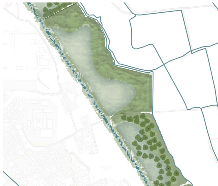
Figure 4.13: The canals in the hinterlands are connected to adjacent areas which are transformed to wetlands and alluvial forests to slow down water and increase infiltration rates
