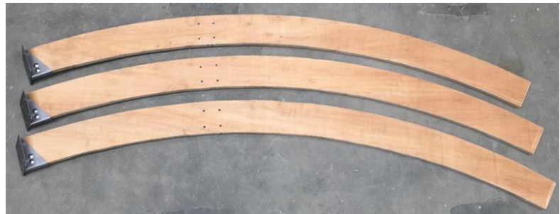
Figure 15. The prototype of the Type 60° connection system connected to the beams.
