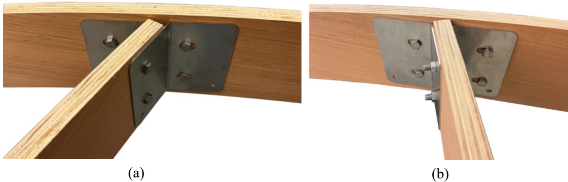
Figure 10. Second version of the connection system (a) Type 60^\circ and (b) Type 108^\circ on prototype scale.
