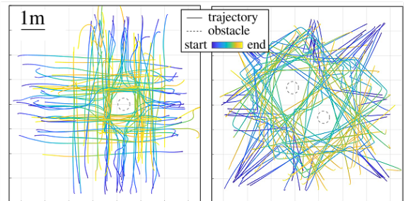
Figure 3: Examples of trajectories including one (left) and two (right) obstacles. These trajectories show the coordinates of the manually controlled MAV provided by OptiTrack.
