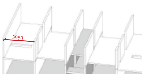
Figure 9. Load-bearing system of Inter-vam flats
