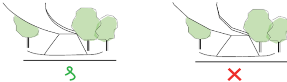
Figure 2.5: Smooth, curved bottom deck edges are preferred over rationalised ones - Requirement by Quality Team
