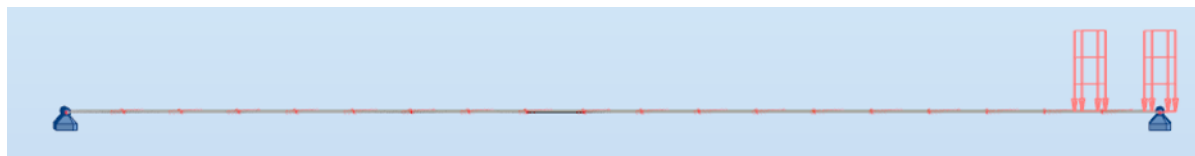
Figure 3.43: TS Loads for Maximum Shear (Longitudinal View) (Robot Model)
