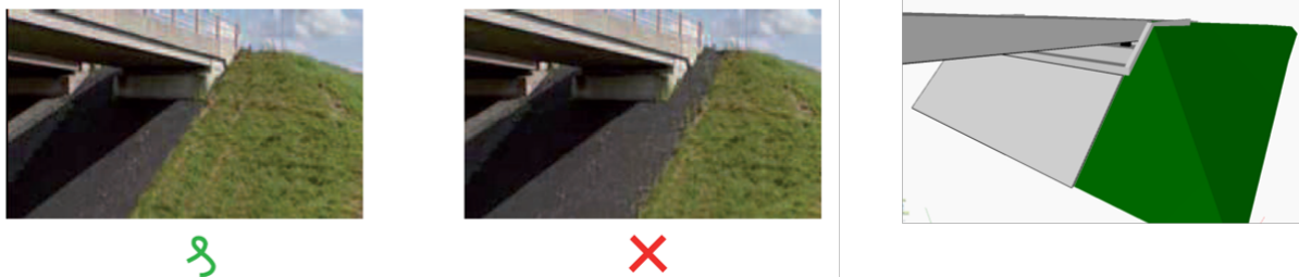
Figure 4.4: (a) Desired abutment design (b) Unwanted abutment design (c) Abutment modelled in Dynamo
