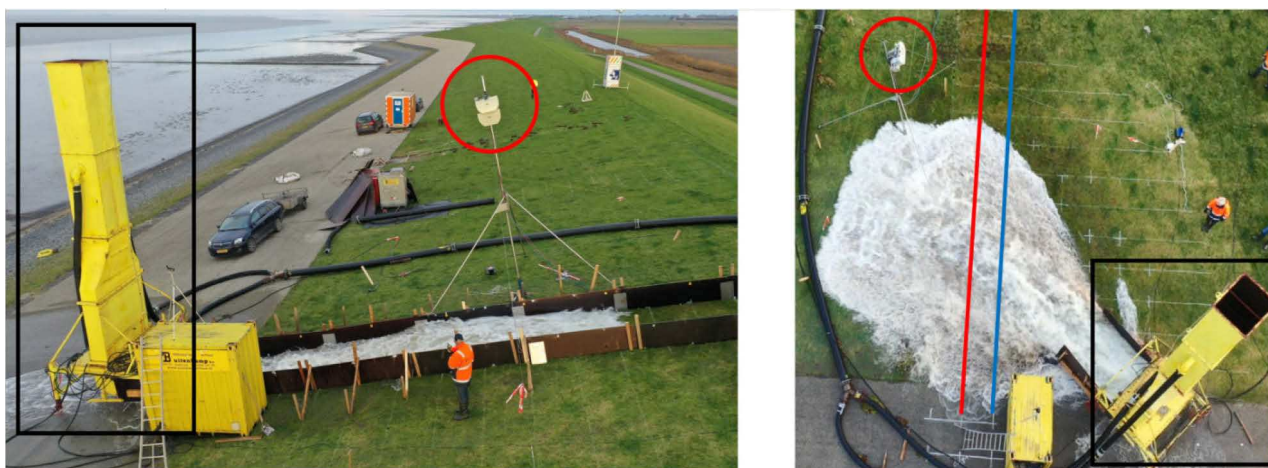
Fig. 1. Left: Laser scanner system (red circle) and run-up simulator (black rectangle) during tests with normally incident waves. Right: Top view during obliquely incident waves (scan lines indicated by red and blue lines).
