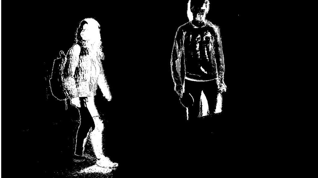
Figure 3.4: Background subtraction. The more white pixels there are the more activity there is on the frame. Therefore for the activity, the amount of white pixels is counted.
