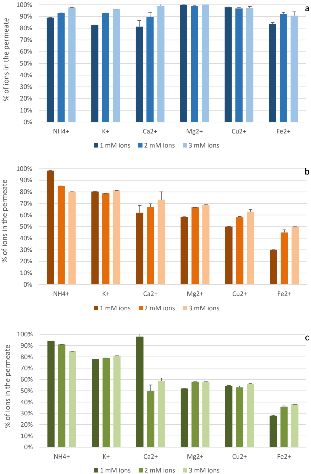
Figure 8: Melanoidins-metal complexation at (a) 0 mM melanoidins, (b) 10 mM melanoidins and (c) 20 mM melanoidins with initial ions concentrations of 1mM, 2mM and 3mM presented as the percentage of ions concentration in permeate compared to initial ion concentration. Bars indicate standard errors (n = 3)
