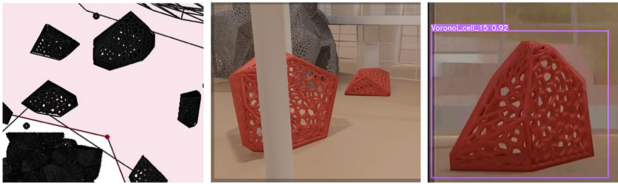
FIGURE 6 Random camera and components distribution within the 3D model of library (top view left), an example input image from the setting (middle), and object recognition (right) implemented via an app on the phone.
