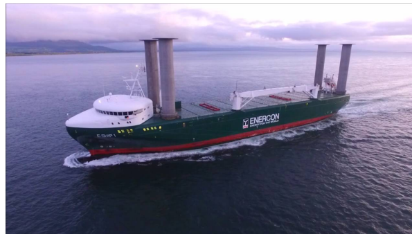
Figure 4.24: Wind assistance: Flettner rotors (McKenna, 2016)
