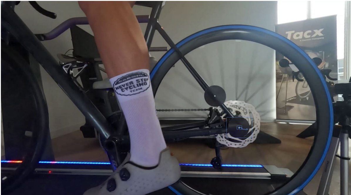
Figure (3.2) The markers for motion tracking on the rear wheel axis and seat stay to determine the longitudinal motion of the bicycle during treadmill cycling.
