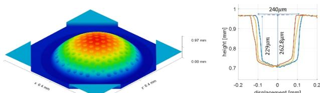
**Fig. 3.** Measured 3D profiles of the core-lens prototype and 2D profile of the center hole.
