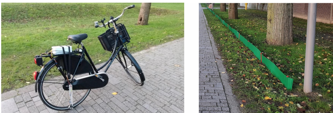
Fig. 4. The instrumented bicycle used for the experiment (left) and barrier for measuring lateral position by LIDAR (right).
