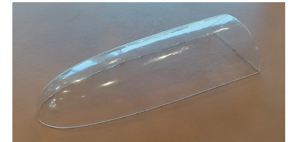
Figure 10.1: Thermoformed PETG product from which the material samples were cut.
