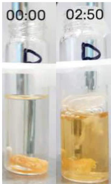
Video 1 –PISOX C at different times during the timelapse experiment. After 2:50 hours PISOX did not completely hydrolyze and dissolve.
