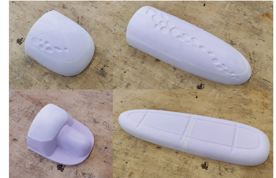
Figure 11.1: The moulds used for thermoforming.
