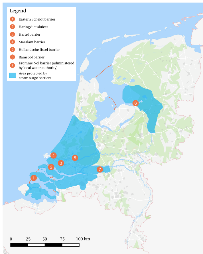
Figure A.1: Parts of the Netherlands for which the storm surge barriers provide flood protection, adapted from Rijkswaterstaat (2018b).
