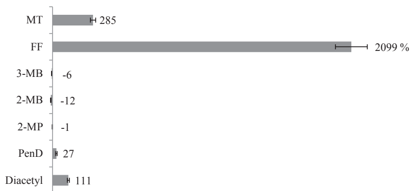
Figure 3.6: Relative increase of aldehydes and diketones during dealcoholisation of Glucose/Ribose-mix obtained from mass balance
