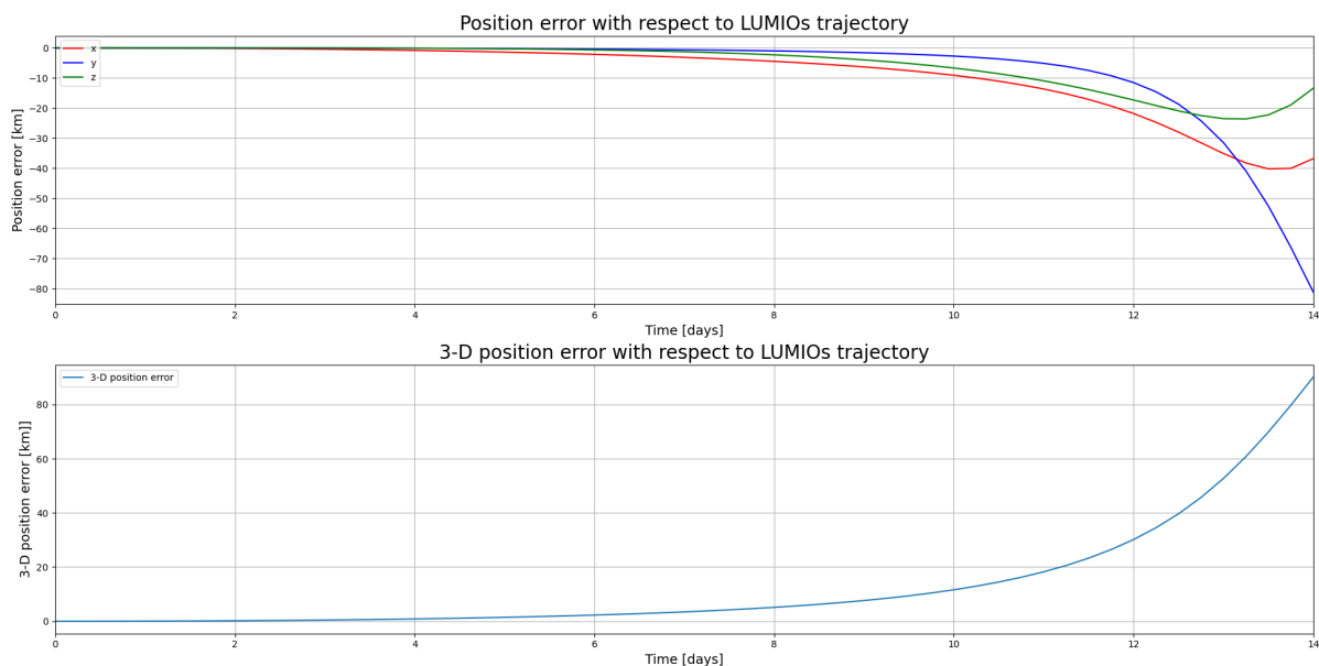
Figure 3.2: Position error of the dynamic model with respect to LUMIOs planned trajectory.
