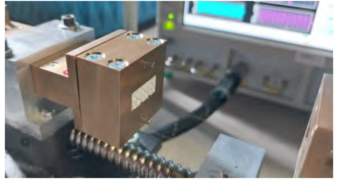
Fig. 6. Rectangular waveguide measurement setup for effective permittivity measurement.
