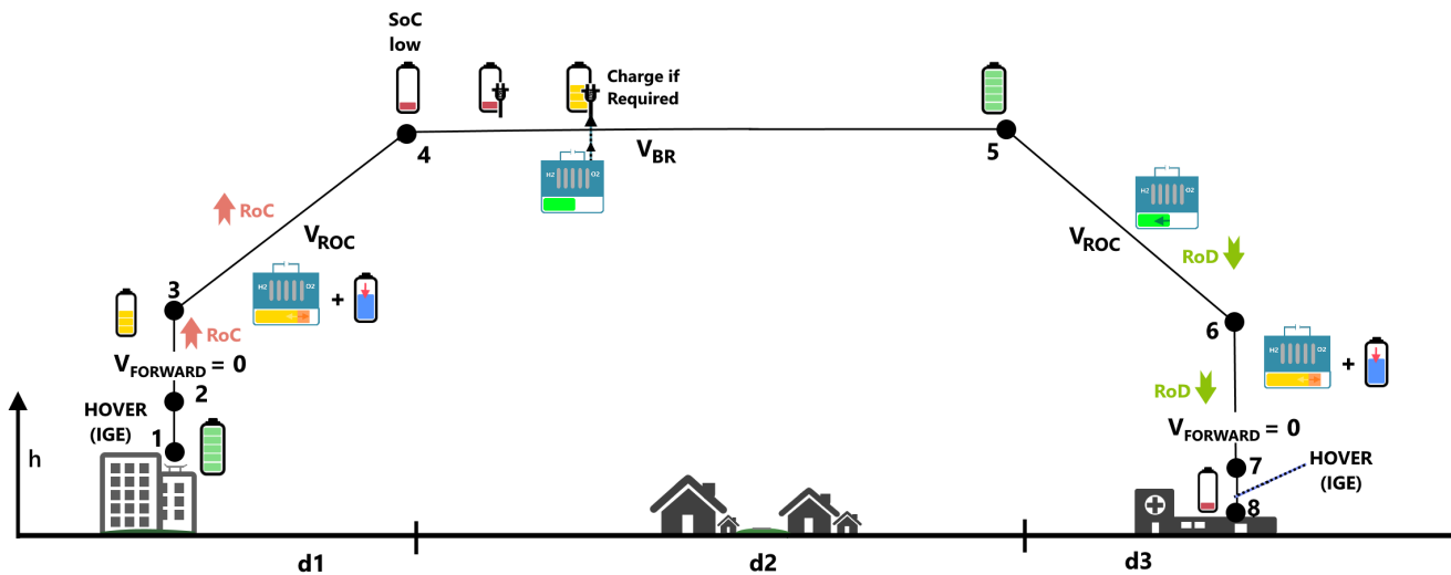
Figure 7.5: Standard mission profile for maximized range (hence V_{br} ) with no intermediate stops.
