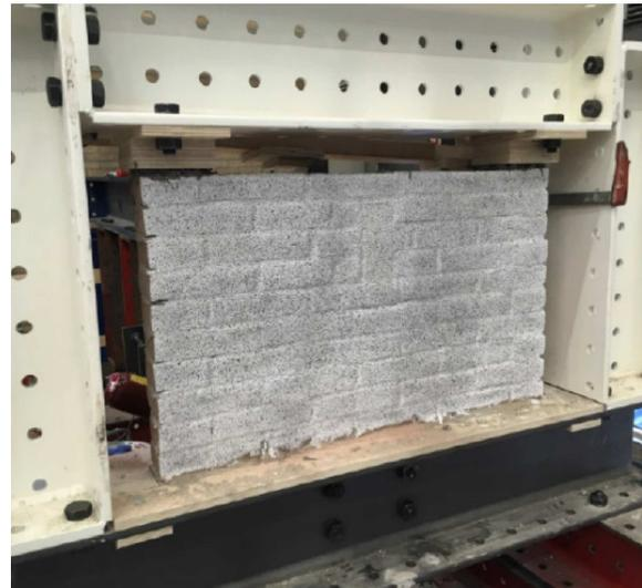
**Figure 4:** Pattern applied to the wall for digital image correlation technique
