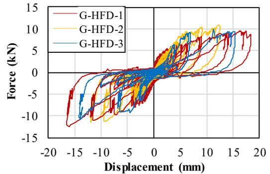
Figure 19: Dynamic response of configuration G
