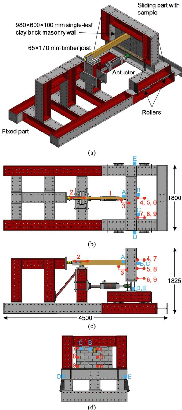
**Figure 3:** Test setup and measurement plan: 3D view (a), plan view (b), side view (c), front view (d); dimensions in mm
