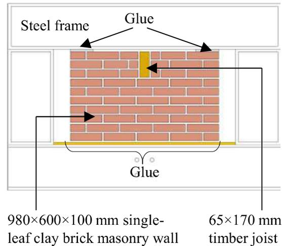
**Figure 1:** Tested timber-masonry connections (A-G) and typical specimen's configuration, including boundary conditions
