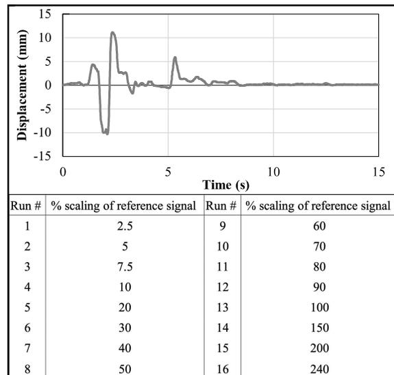
**Figure 2:** Reference signal adopted for high-frequency dynamic tests; the various runs and their amplitudes are also shown
