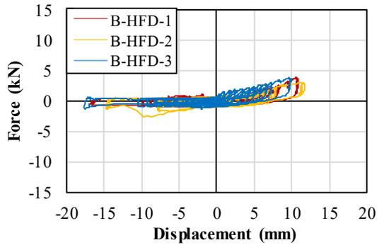
Figure 14: Dynamic response of configuration B
