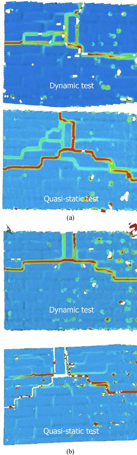
**Figure 20:** Comparison between the crack pattern observed at the displacement corresponding to peak force for dynamic and quasi-static tests in configuration E (a) and F (b)
