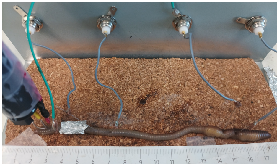
Figure 22: Close up view of the worm in the Faraday cage before an experiment involving magnetic and tactile stimulation.
