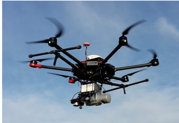
Figure 1.2: The drone in action: The UAV of Shore Monitoring and Research equipped with a camera, positioning system (GNSS), motion sensor (IMU) and LiDAR in action. (see section 3.2.2 for further elaboration)
