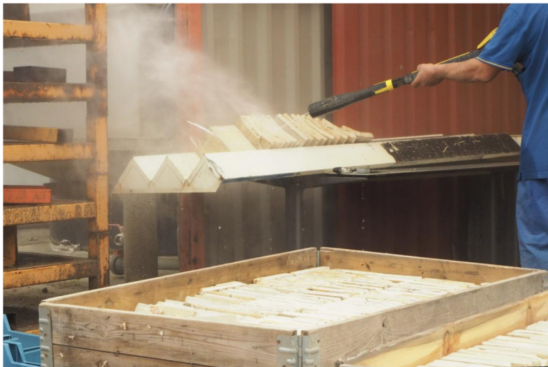
cleaning of reclaimed ceramic tiles © RotorDC
