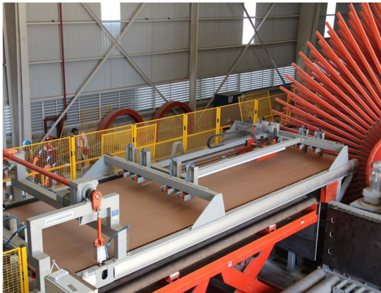
MDF board production - cutting process © Woodworking Network
