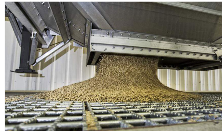
MDF board production - adding resin © Action Tesa
