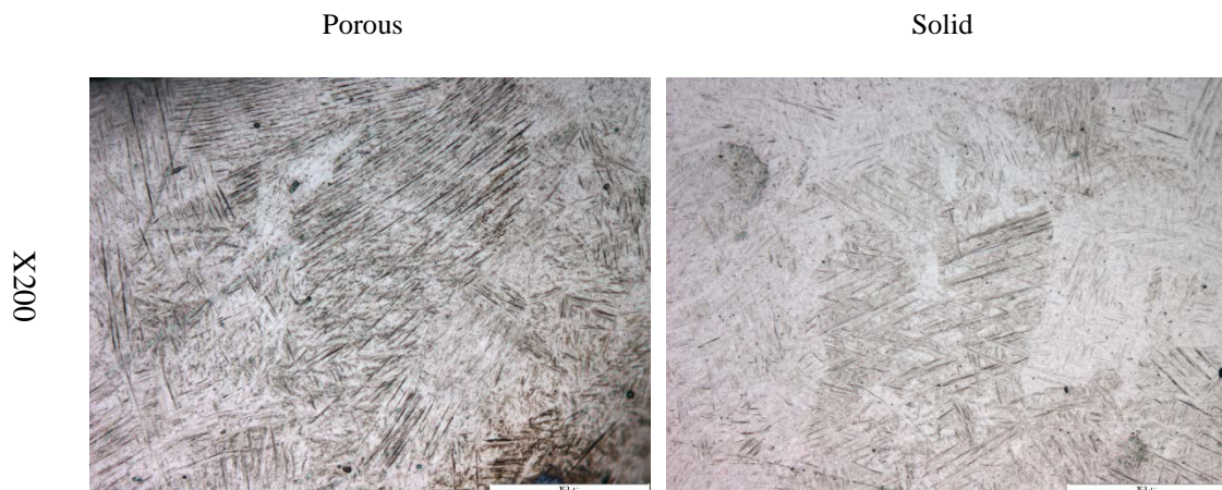
Figure 7-5. SEM picture of the microstructure of additively manufactured (a) Ti-6Al-4V, (b) Co-Cr porous structures with etched cross-sections
