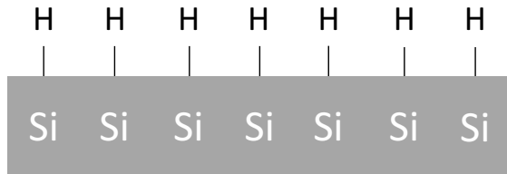
Figure 3.2: Simplified view of the Si substrate without the native oxides after treatment with HF. Hydrogen has bonded to the surface of the Si.
