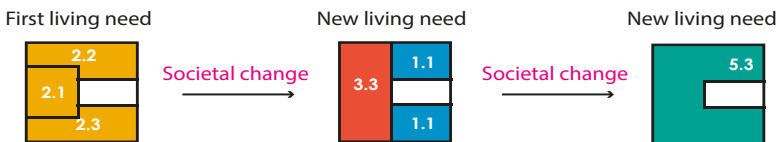
The way the cube is designed also makes it possible to choose the distribution Figure 30: The possibility to change the Bremer Punkt due to the change in society. Drawing by Author. (Lemnawar, 2022)
