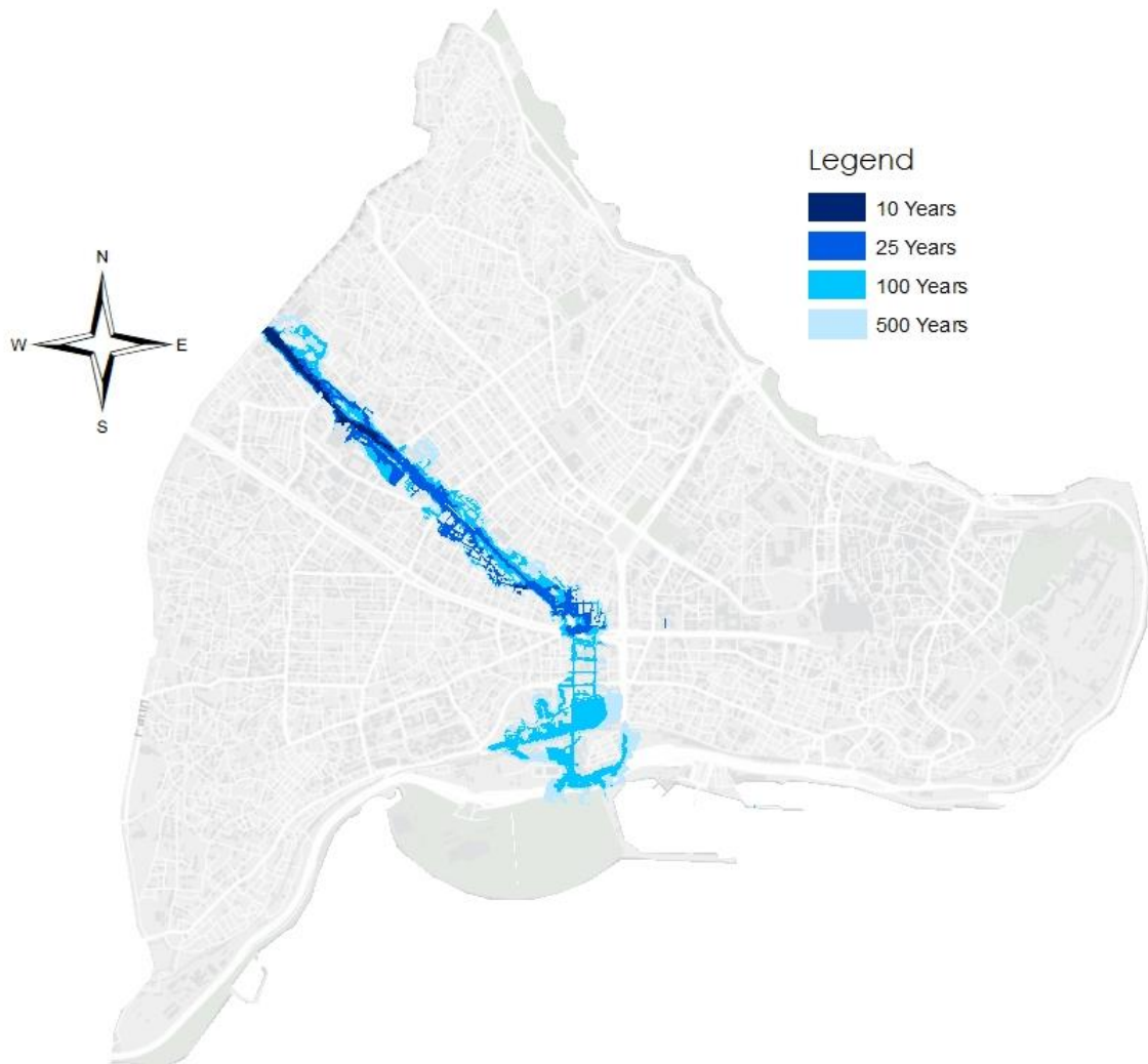
Figure 8: Flood sensitivity map of the Lykos watershed provided by AKOM on behalf of ISKI visualised in ArcGIS. The numbers in the Legend refer to return periods.
