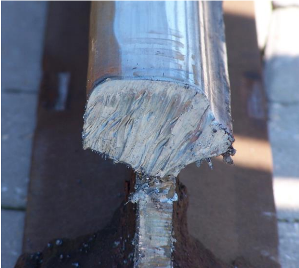
Fig. 8. severe wear and downward plastic flow at the rail gauge corner
