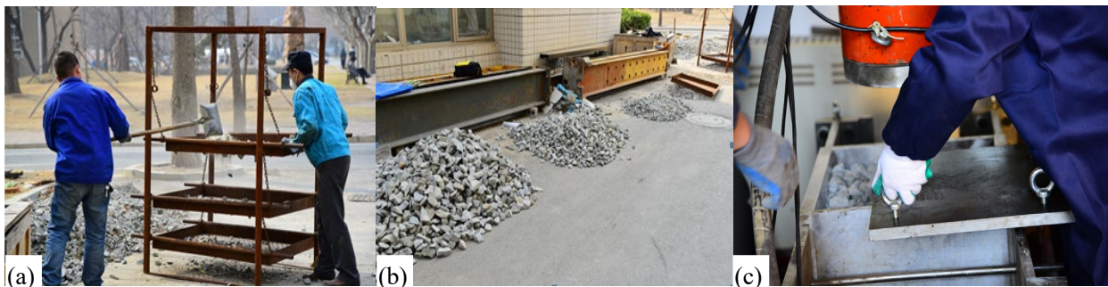
Fig. 12 Overview of the shear test preparation: (a) screening ballast; (b) classifying ballast; (c) loading ballast
